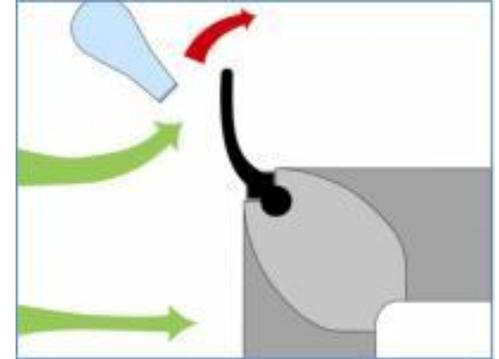
The greatest air flow rates are achieved when the ACTIVLOUVRE system is fully open but, with the ability to vary its position to control the ventilation rate, the louvres can be closed to prevent the ingress of heavy rain and snow.
