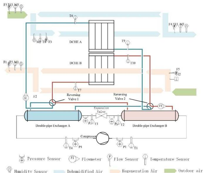
**Fig 2** – Schematic diagram of the Novel AHU
