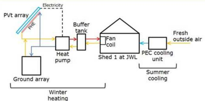
Fig 1 – WelChic system schematic
