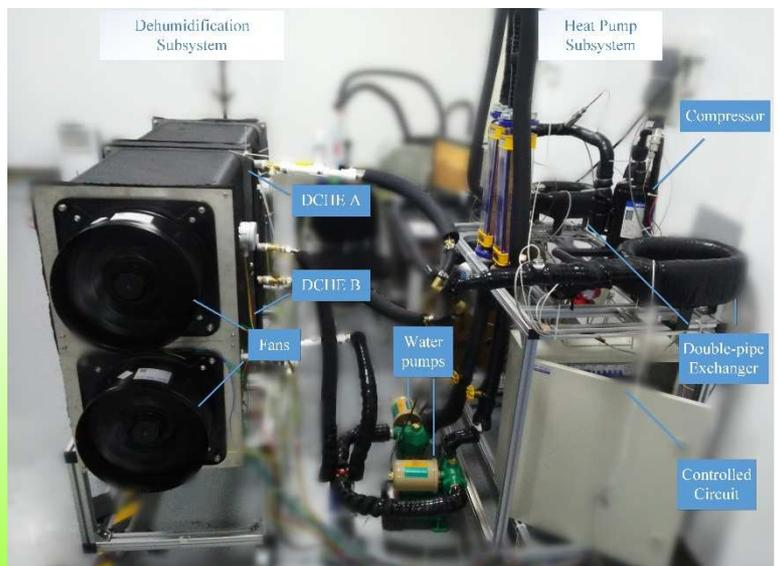
**Fig 1** – Air handling unit with dehumidification by desiccant coated heat exchanger
