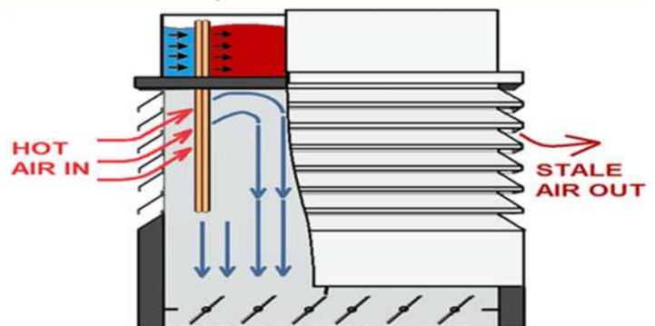
**Fig 1** – Operation schematic of the multi-direction passive cooling wind tower
