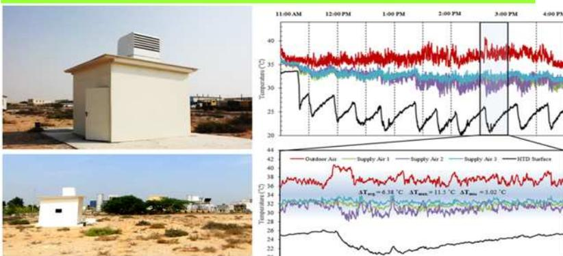
**Fig 2** – Test site located in Ras Al Khaimah, to test the temperature drop using the uni-free wind tower
